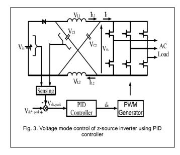
The modified pulse width modulation is employed here to achieve shoot through state. It can be understood as using the following figures
