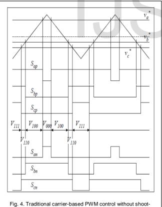
through zero states, where the traditional zero states (vectors) V111 and V000 are generated every switching cycle and determined by the references The switching method which produces shoot-through state is shown in the following figure which can be easily understood.
